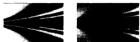
( F_n=0.00 ) ( F_n=2.91 ) Fig. 14 Wave pattern at F_n=0.75
