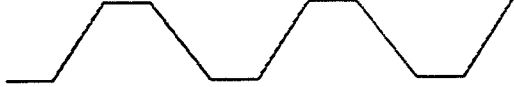
Fig. 3 Configuration of the bent copper wire for fabrication of a Kagomé core
