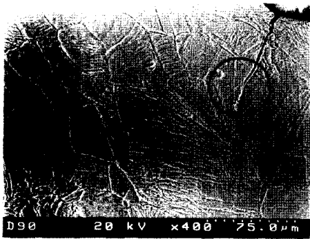
(a) Crack propagation(x400)
