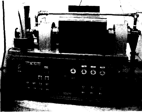
Fig. 2 Photography of the rotary kiln used at pyrolysis and firing.
