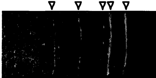
Fig. 19 Distributions of electro-rheological particles for Re=0.62 along the test tube with D.C 1.5kV/mm.
