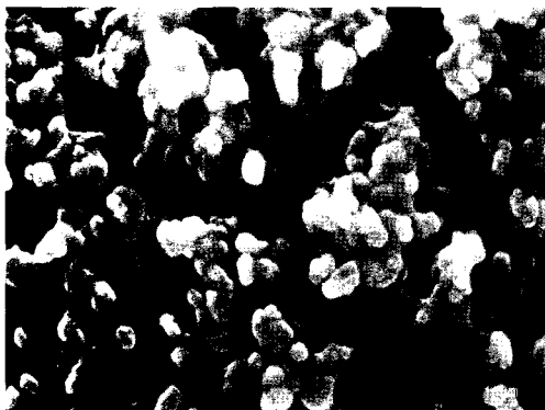
Figure 7. SEM photograph of PVAc nanoparticles containing erythromycin.
