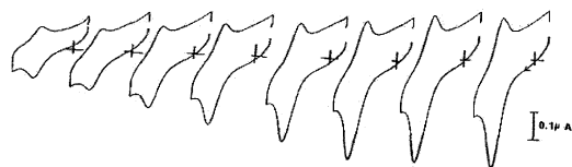
Fig. 2. CV responses at 10 mV/s for Au/cys-dopa electrode in 0.1 M phosphate buffer(pH=7.10) as a function of NADH concentration: none, 0.114, 0.337, 0.662, 1.08, 1.58, 2.06 and 2.52 mM.
