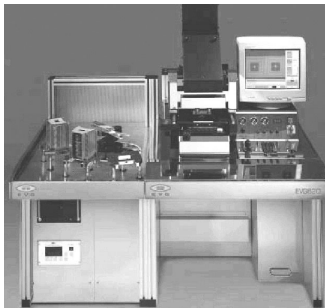
그림1. EVG 620 imprinting lithography equipment
