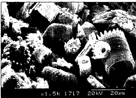
Fig. 8. Cylinder shaped diatomaceous earth observed in Kromafaze commercial alginate impression material ( \times 1500 ).
