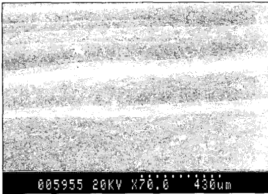
Fig. 11. Paladent ® 20 with POSS : SEM photograph of abraded surface with toothpaste solution at magnification of 70X.
