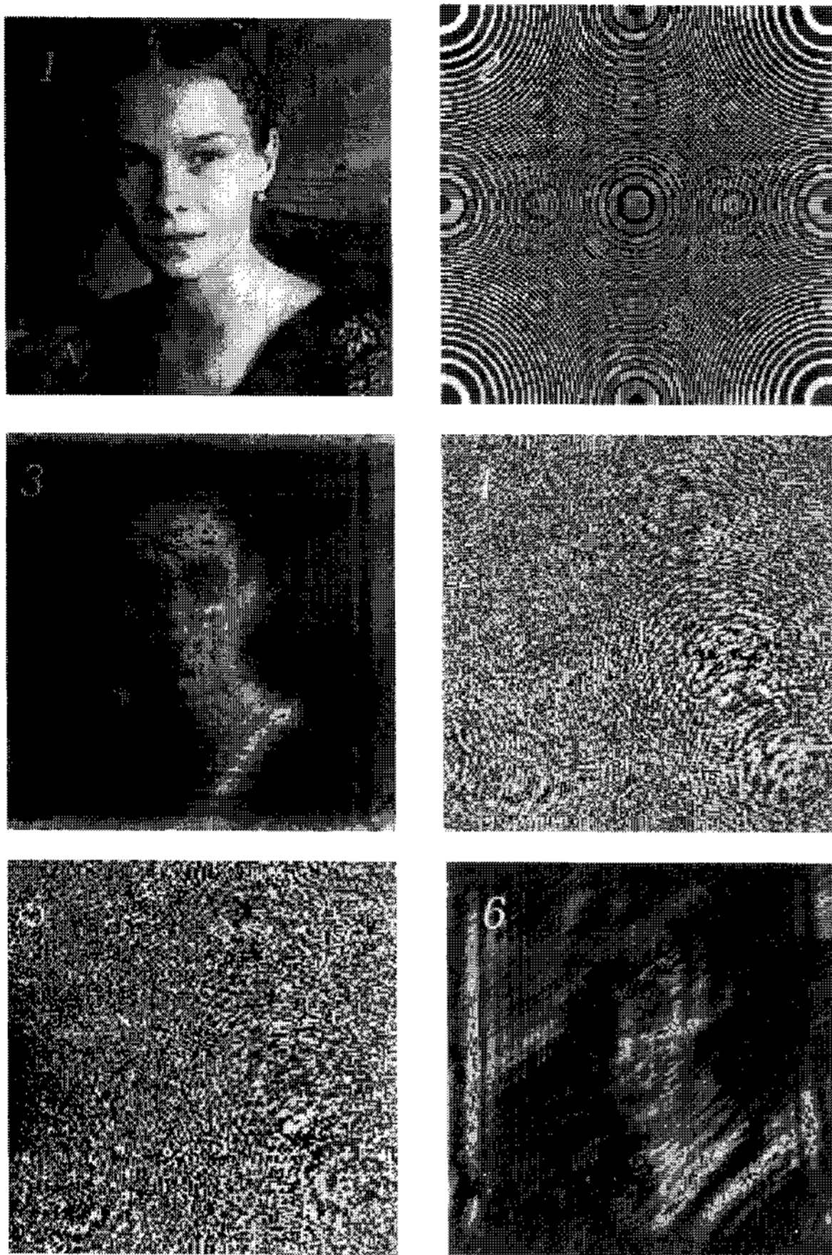
Fig. 3. Optical image holographic recording and toelectrical signals transformation illustration. 1) one plane of 3-D object; 2) convolution corn function; 3) object's optical hologram; 4) Fourier-image of optical hologram; 5) this Fourier-image after coordinates transformation; 6) electrical signals field.
