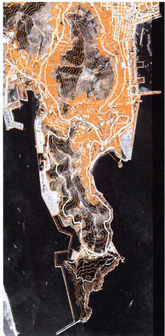
Fig. 1. An integrated digital database for SeoGu, Busan by overlay of KVR-1000 satellite image, DTM and ENC
