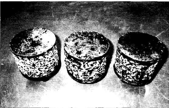
그림 6. Debonding between the waterproofing membrane and the concrete (Sheet types)
