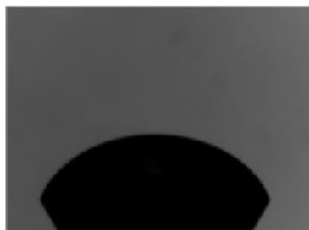
Figure 2. A typical image of a sessile drop (DER 664 UE at 166 °C) on top of a stainless-steel cylinder reproduced by a laser printer. From this profile, ADSA determines the surface tension to be 38.14 \pm 0.26 mJ/m 2 .
