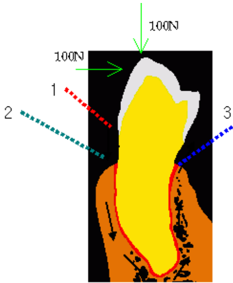
Fig. 7. A Path along which calculated von mises equivalent stress were compared. number 1 in figure indicates labial CEJ, number2 indicates root surface at buccal bone crest level. And number 3 indicates root surface at lingual bone crest level
