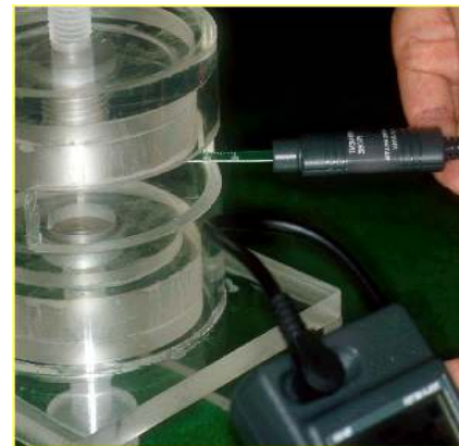
Fig. 3. Evaluation of strength of magnetic field with Gauss meter
