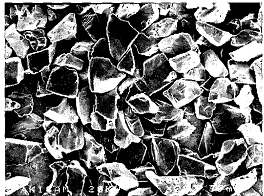
Fig. 10. SEM photograph for the SiC powder synthesized at 1600°C for 120 minutes material of SiC+Si and C.
