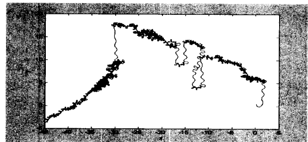
Fig. 7. Trajectory of the mobile robot of Chua's equation ,when there is no boundary
