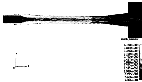
Fig. 4 Mach number distribution with secondary duct radius 15mm
