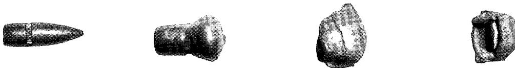
Fig. 14 A deformation of 5.56mm ball projectile by high velocity striking
