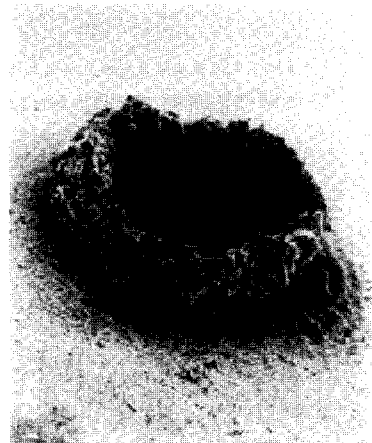
Fig. 2. Laser ablated crater in Zn based alloy surface with the use of 6ns pulse from a Nd:YAG laser at 532 nm.
