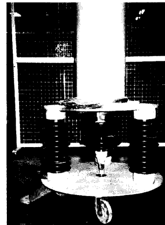
Fig. 4 Mounting DSS insulator under impulse puncture test in air
