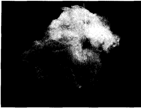
Fig. 4. External appearance of the kenaf fibers retted chemically after removing non-cellulose.
