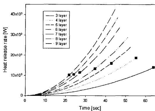
Fig. 5. Heat release rate vs. activation time of detector (for rate of rise).
