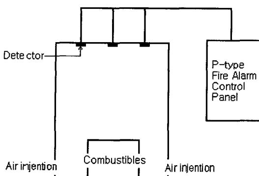
Fig. 3. Schematic of experimental setup for fire simulation.
