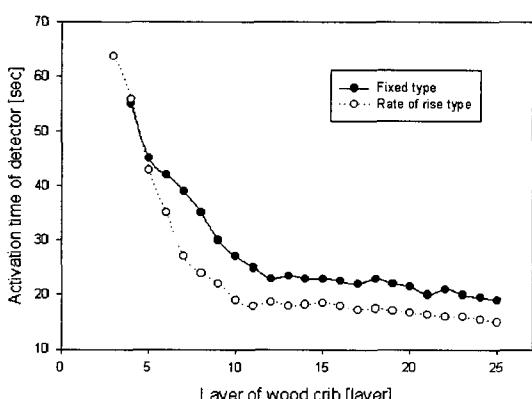
Fig. 4. Activation time of detector vs. the layer in the wood crib.
