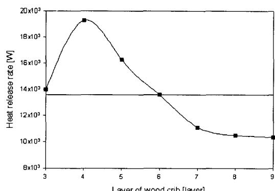
Fig. 6. HRR to activate detector vs. the layer of wood crib (for rate of rise type).
