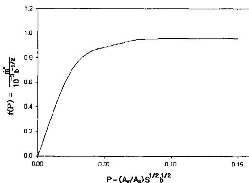
Fig. 2. The reduced specific burning rate.
