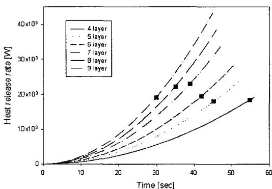
Fig. 7. Heat release rate vs. activation time of detector (for fixed type).
