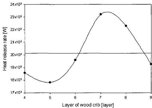
Fig. 8. HRR to activate detector vs. the layer of wood crib (for fixed type).
