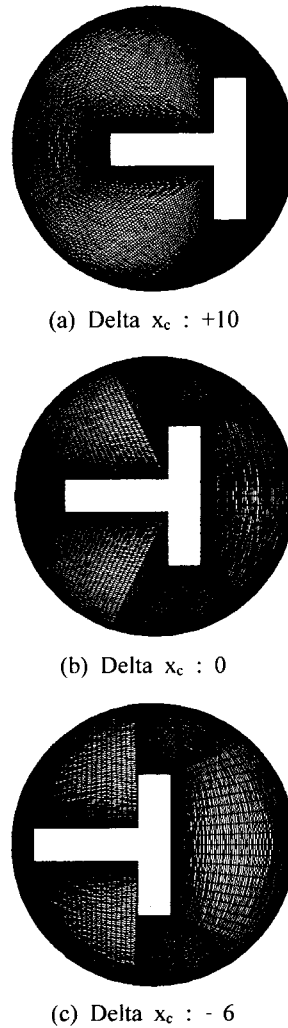
Fig. 14 Variation of the generated die surfaces obtained by moving the center point
