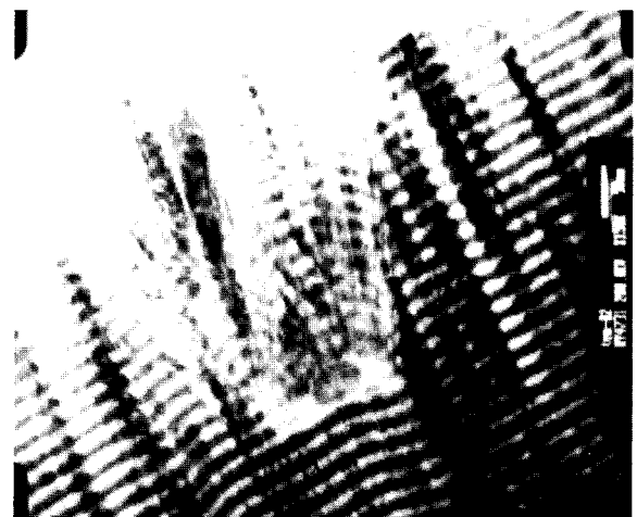
Fig. 5. Cross-sectional electron micrograph of droplet embedded in multilayered coatings.
