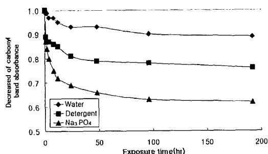
Fig. 2. Decrease of carbonyl band absorbance of cotton fabric treated with DMDHEU and hydrolyzed in different solution at 70°C.
