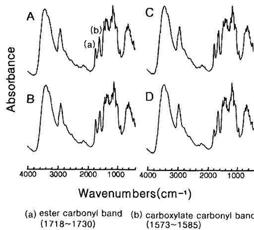
Fig. 3. Phtoacoustic infrared spectra of cotton fabric finished with polycarboxylic acid (A) MA, (B)CA, (C)BTCA, (D)PMA.
