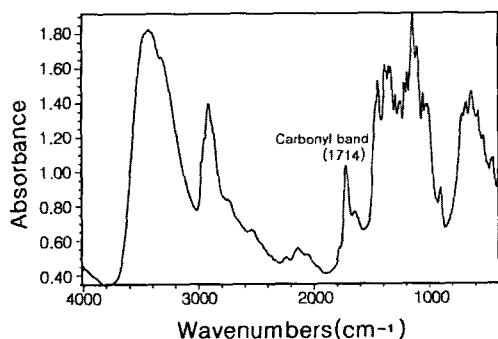
Fig. 1. Phtoacoustic infrared spectra of cotton fabric finished with DMHDEU.
