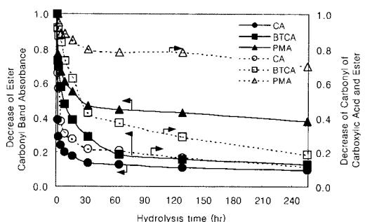
Fig. 7. Decrease of ester carbonyl, and carboxylic acid and ester absorbance of cotton fabric treated with carboxylic acid and hydrolyzed in 2% NaOH solution at 70°C.
