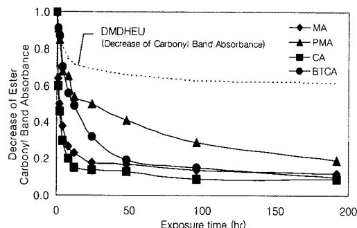
Fig. 6. Decrease of ester carbonyl band absorbance of cotton fabric treated with carboxylic acid and hydrolyzed in 1% Na<sub>3</sub>PO<sub>4</sub> solution at 70°C.
