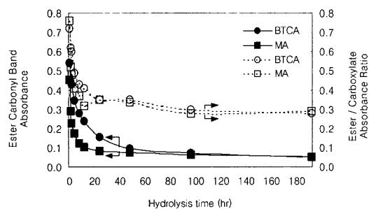
Fig. 10. Ester carbonyl band absorbance and carbonyl band intensity ratio of cotton fabric treated with carboxylic acid and hydrolyzed in 2% NaOH solution at 70°C.
