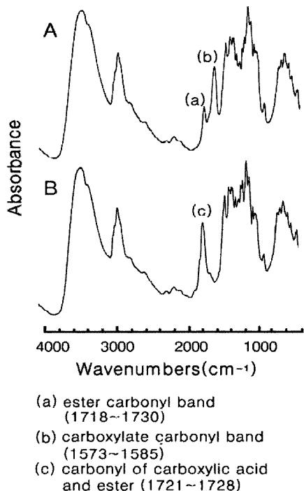
Fig. 8. Infrared spectra of cotton fabric treated with PMA. (A)treated with an 0.1M NaOH (B)treated with an 0.1M HCl (C)carbonyl of carboxylic acid and ester.
