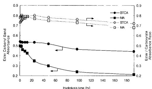
Fig. 9. Ester carbonyl band absorbance and carbonyl band intensity ratio of cotton fabric treated with carboxylic acid and hydrolyzed in deionized water at 70°C.
