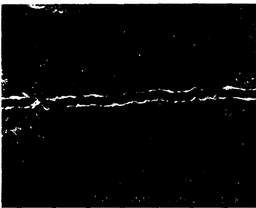
(b) Macro cracking
