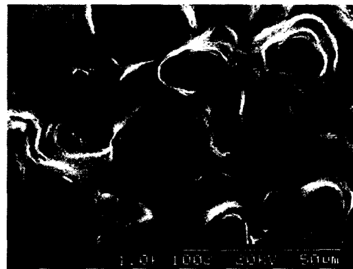
Fig. 7 SEM fractograph of oxidized solidification crack morphology
