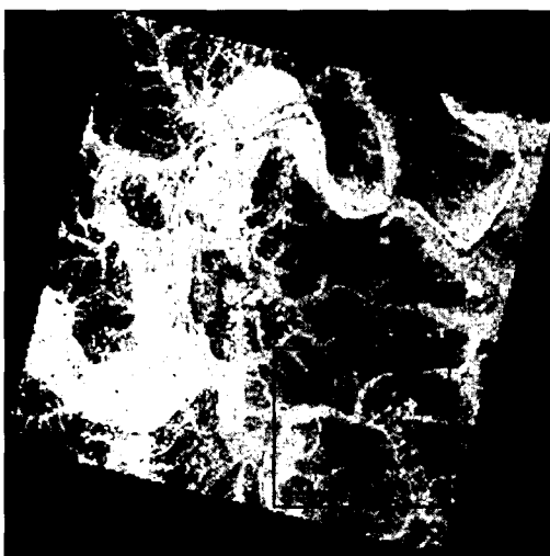
Fig. 1. Geometric correction image of the stereo pair and area for the DEM generation (Image size: 1200×1200 pixels).
