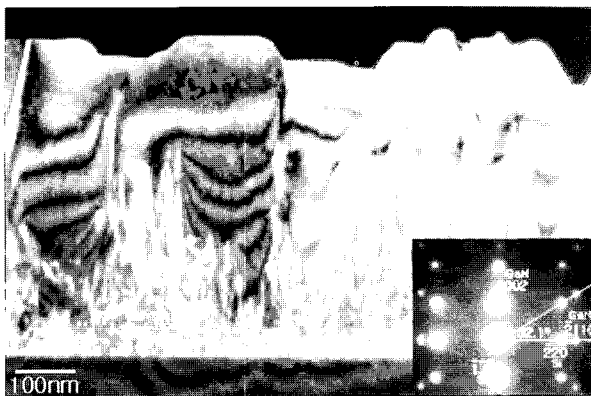
Fig. 5. A cross-sectional TEM dark field image of 1,000°C GaN/LT-GaN/AlN/Si specimen. The image using the diffracted beams of g = 0002 . Inset is a SADP taken from GaN/LT-GaN/AlN/Si. The diffraction pattern consists of Si zone axis pattern and GaN zone axis pattern.
