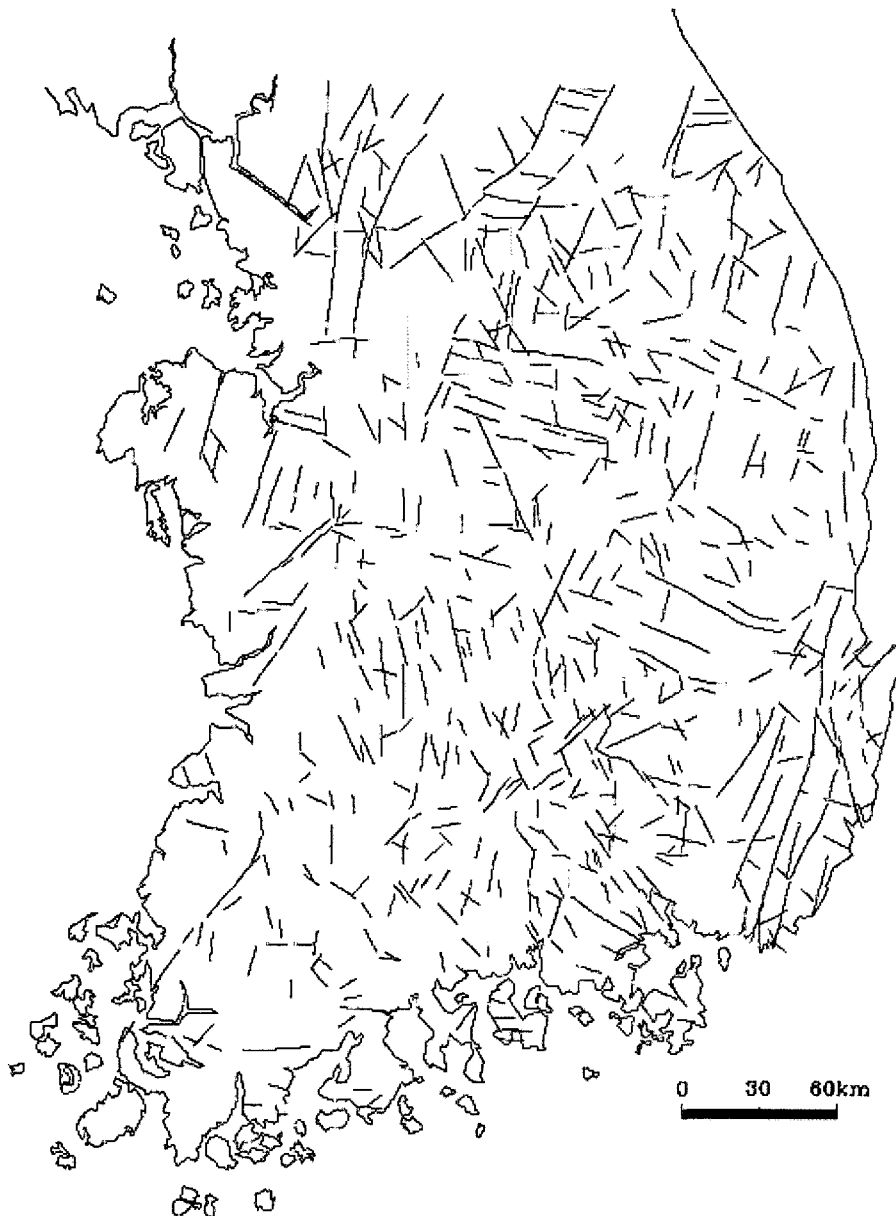
Fig. 2. Lineaments interpreted from shaded relief maps of 1 : 250,000 and 1 : 500,000 scales.
