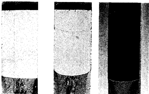
Un-peening(RT) Shot-peening(RT) Shot-peening(180°C) Photo. 1 Photographs of fracture surface
