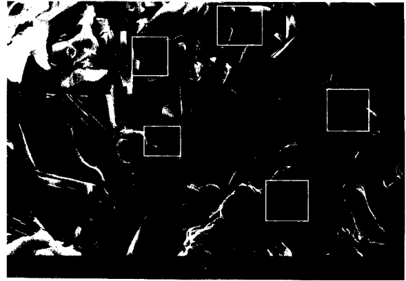
Fig. 5. Scanning electron micrograph(5000 times) of the surface of TI-III film.
