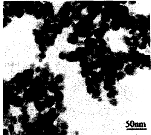
Fig. 2. CoFe 2 O 4 nanopowders synthesized by MCP from FeCl 3 +CoCl 2 +NaOH mixture.
