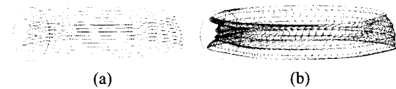
Fig. 1 Vertical shape inconsistency between contours; (a) Contour data with noise, (b) Wiggled surface
