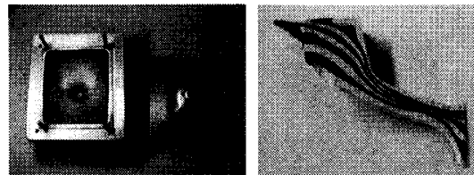
Fig. 13 Semi-metallic soft mold and results of CRT forging test
