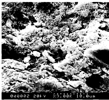
Fig. 7 A SEM photomicrograph for cross-sectional view of test piece (admixture added)
