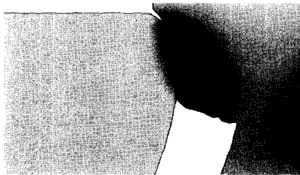
Fig. 3 Folding initiation by small fillet angle( 45° ) of moving die and inserts initiation
