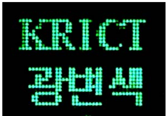
Fig. 6. Reconstruction of an image stored by spatial light modulator in the photochromic film. (pixel size : 42 \mu m)
