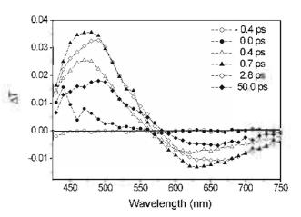
**Figure 3.** Time-resolved transient transmittance spectra of 1-HAQ in toluene with varying the delay times from -0.4 to 50.0 ps. The excitation wavelength was set to be 405 nm. The polarization between pump and probe beam was set to be a magic angle configuration.
