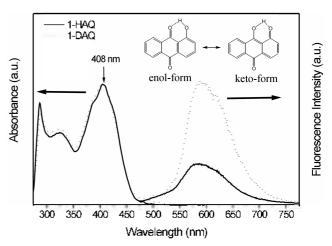
**Figure 1.** Absorption and emission spectra of 1-HAQ (solid lines) and 1-DAQ (dashed lines) in toluene at room temperature. The excitation wavelength for the emission spectra was set to be 408 nm, which is the absorption maximum of the two anthraquinone derivatives. The emission spectra were observed under the same experimental conditions such as optical densities, excitation wavelength and detection sensitivity for the two anthraquinone derivatives.
