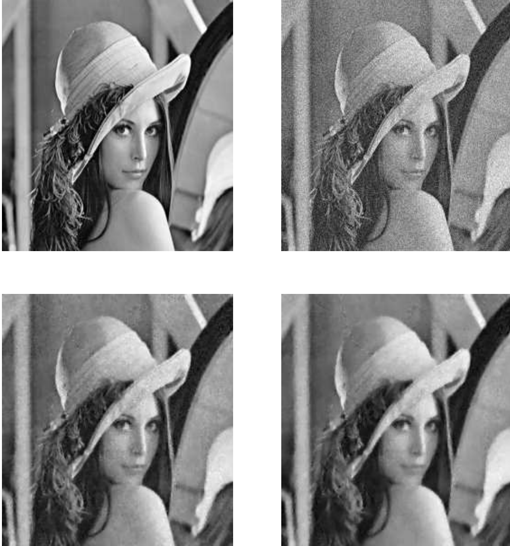
FIGURE 5. (a) Upper left is original Lena Image. (b) upper right is noisy image with Gaussian noise of \sigma = 20 . (c) Lower left is denoising image with optimal values \alpha = 3 \times 10^{-2} , \beta = 10^{-6} in L^2 norm sense. (d) Lower right is denoising image with optimal values \alpha = 5.5 \times 10^{-2} , \beta = 10^{-6} in H^1 norm sense.
