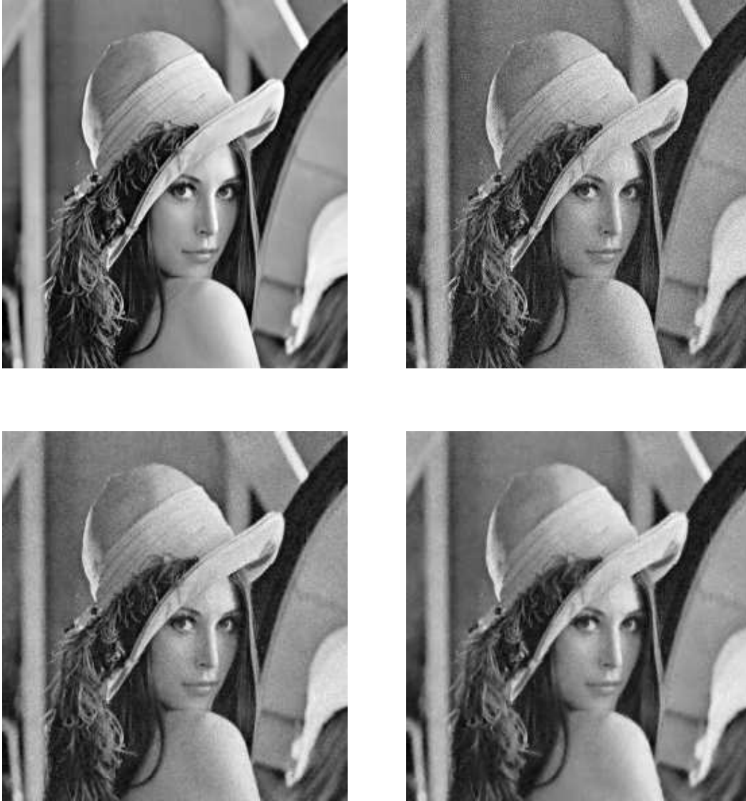
FIGURE 4. (a)Upper left is original Lena Image. (b)Upper right is noisy image with Gaussian noise of \sigma = 10 . (c)Lower left is denoising image with optimal values \alpha = 6.5 \times 10^{-3} , \beta = 10^{-6} in L^2 norm sense. (d)Lower right is denoising image with optimal values \alpha = 15.5 \times 10^{-3} , \beta = 10^{-6} in H^1 norm sense.
