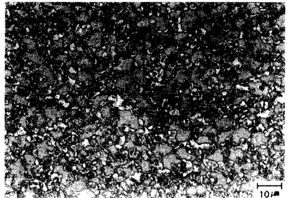
Fig. 8. Optical microscopy of color etched HSLA-100 steel after aging at 620°C.
