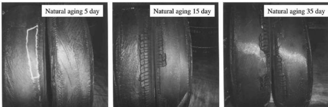
Figure 8. Fracture surface of steel belted layer after tire endurance testing.
