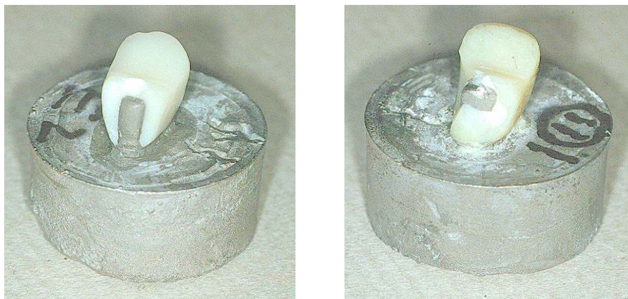
Fig 4. Fractured surface of IPS-Empress(left) and Targis(right) crown. The fracture line of crown began at the loading point and extended along long axis of tooth. IPS-Empress showed adhesive failure pattern whereas Targis had adhesive and cohesive failure.
