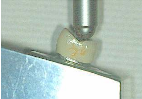
Fig 1. Diagram shows the loading point that is middle on the buccal incline of lingual cusp. 15°angulation between crown and loading stylus on the universal testing machine.
