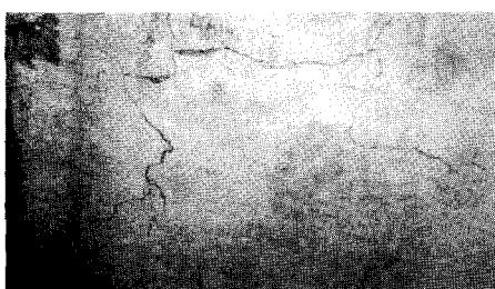
Fig. 12 Failure pattern at the bottom surface (bonded case)
