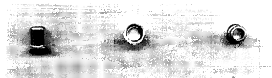
Fig. 5 Specimens used in the barrel electroplating experiment
