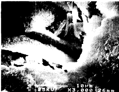
사진 2. Attached fiber in cement matrix.
