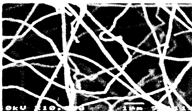
Figure 8. SEM image of as grown Pyrograf™-III carbon nanofibres (Courtesy: Pyrograf Products, Inc. USA).
