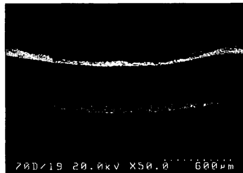
Fig. 9 Shape of oxide film (F.Z & PMZ)
