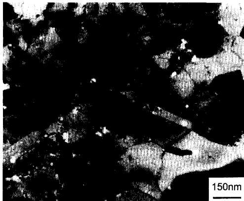
Fig. 4. TEM micrograph of a Cu-3vol.-% TiC in-situ alloy ( d_{Cu} \approx 200\text{ nm} ).
