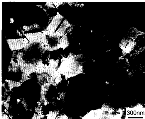
Fig. 5. TEM micrograph of a Cu-3vol.-% TiC powder alloy ( d_{Cu} \approx 400\text{ nm} ).
